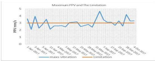
Figure 4. Maximum vibration and limitation
